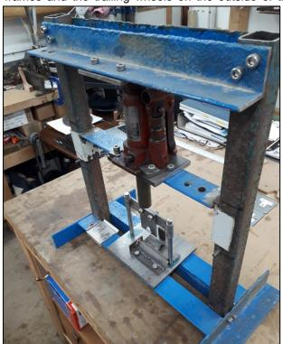
frames have to be bent and to make a tidy job of this I constructed a bottle jack press from an old car jack I had under the bench and the remains of a glider trailer. I also made up a press tool with fence and depth stop so I could ensure repeatability with each bend.
