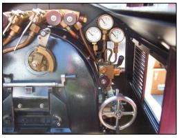
building the was locomotive in 7 1/4." This locomotive was a traditional mallet with the four cylinders compounded in two pairs. The 3'6" gauge prototype was built in 1920's in Holland. The attention to detail on the model was stunning with fully working scale controls, including vacuum brake. This was complimented by a working tender water gauge (pointer around a semicircle). re-railing jacks and
