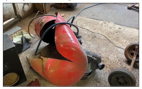
Also, on this You Tube page on the right-hand side there are a number of other videos where a similar catastrophic failure of the air tank has occurred.
