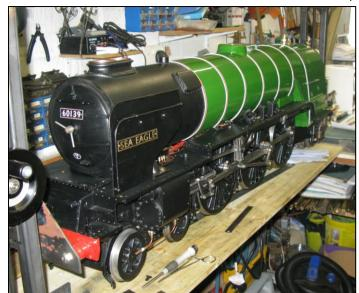
rails have to be done, the steam exhaust pipe from the ejector to the smoke box, the drain cock rods from cab to the front and safety valves have to be completed.
