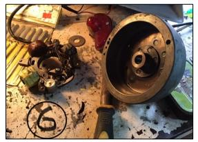
have taken photos of the wheels before the spokes removal to help me install the new. I have cleaned the points, (photos6&7) and on hand spinning the generator flywheel I got a good spark, so it bodes well for starting up. I am now sourcing the paint and the four cables, (clutch, front brake, gearbox and accelerator.) I have already got the two new tyres and inner tubes as the existing ones had
