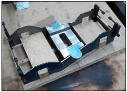
These had to be bent so that the axis of the central hole was perpendicular to the longitudinal axis of the bogie.
