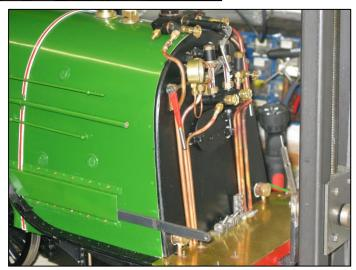
also the tender connecting pipe work to be fitted.
