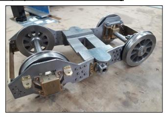
As many will know, the King bogie has the leading wheels on the inside of the frames and the trailing wheels on the outside of the frames. Accordingly, the
